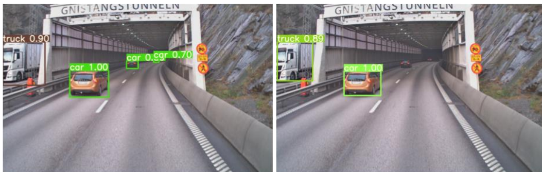
Figure 22: Comparison of YoloV3 detector, trained with the Volvo Dataset and with public data. The left image shows the detector trained with the Volvo dataset. The right image shows the detector trained with public dataset. The second detector is not able to detect the two vehicles at the end of the ego road.
