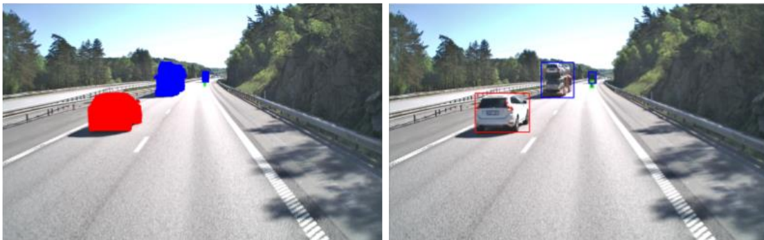
Figure 13: Annotation for Object Detection. The left image contains the mask for object segmentation and the right image contains the bounding boxes for the objects and the object classification.
