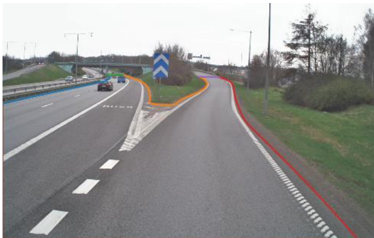
Figure 17: Annotation for road edges with asphalt segments.
