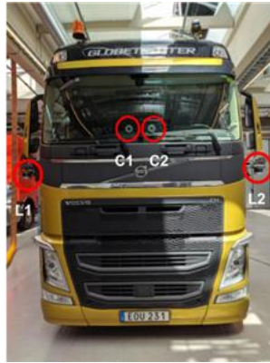
Figure 4: Sensor placement for the logging system in Perception.
